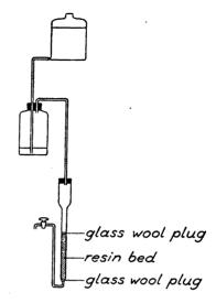
Fig. 1. Ion exchange apparatus.
